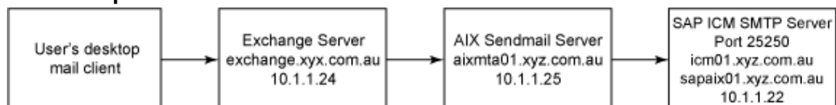
Figure 2. Mail flow from desktop, through Sendmail server, to SAP ICM SMTP server on port 25250
